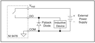
Figure 4. Connecting a Flyback Diode to the NI 9476
